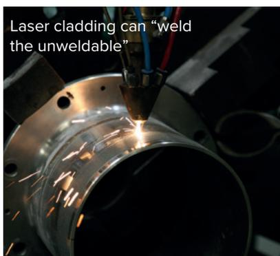
Laser cladding can “weld the unweldable”
