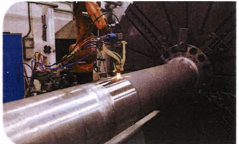
Laser cladding of seal surface
